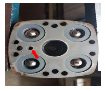
3.5: Apply the sealing compound to the lower half of the fuel distributor. Leave the upper half clamped in the vice.
