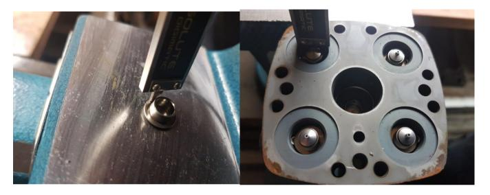
Make a note of the measured values on a small sketch. The values should not be very different. If so, this is an indication that the fuel distributor has been misadjusted or an injector is faulty.
