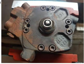
2.5: Loosen the lower part of the fuel distributor from the upper part by short rotating movements of the lower part. If the lower part is stuck, use a hammer to help. Support the short turning movements with light hammer blows on the lower part. When the lower part has come loose, pull it off the upper part. Do not twist the upper and lower parts as this may damage the control cylinder. Never use a screwdriver to pry off the halves. This causes damage to the sealing surfaces.
