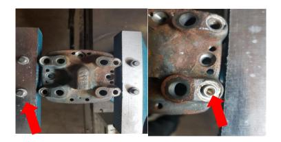
2.9: Unscrew the system pressure regulator on the bottom side of the fuel distributor. Pay attention to the sleeve that may get stuck in the housing.
